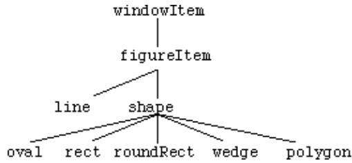
FigureItem is the general superpattern for all vector graphics patterns, implementing the common attributes of all graphics patterns. All figureItems have the attribute pen. Pen is an object used for drawing the figureItem. Pen has attributes for defining the drawing pattern of pen, for defining the foreground and background color of pen, and for defining the size (rectangle) of pen.
